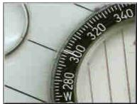
5. In the UK you must add the magnetic variation to the grid bearing to get a magnetic bearing "From grid to mag, add" (this may not be the case in other countries around the world). By adding 5° to the grid bearing at the INDEX LINE gives us a magnetic bearing of 299°.
