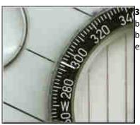
**3.** Take the compass off the map. At the INDEX LINE read the grid bearing. The grid bearing is the angle between the north south grid line and the imaginary line between your start location (Pen Bryn-du) and your destination (Foel-ganol). In this example the grid bearing is 294°.
