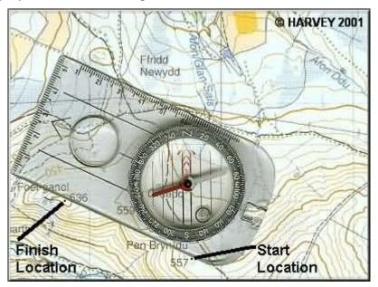
**2.** With the BASE PLATE in this position on the map, turn the COMPASS HOUSING only (not the BASE PLATE) so the ORIENTING ARROW points to the top of the map and the ORIENTING LINES are parallel with the grid lines on the map.
